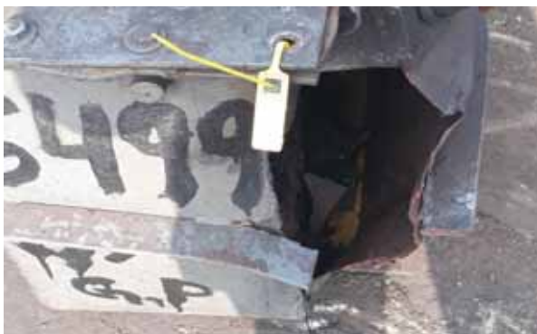
Despite of Explosion vent pipe getting ruptured, PRV operated and DD fuse blowing off as per site report, Tank bulged and bursted
