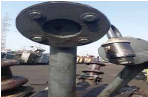
Opening of welding joint from one of the edges breaking stiffener also
